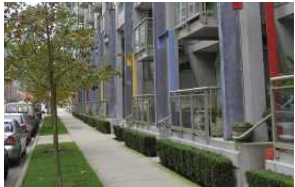
Use alternate height entrances in residential developments with more pedestrian traffic to improve privacy.
