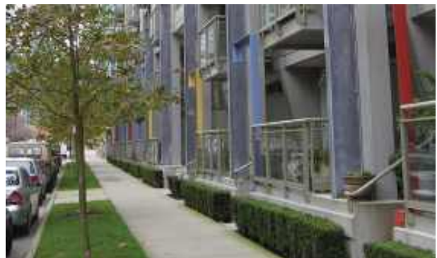
Using grade separated entrances for ground-level residential uses provides privacy for homes while maintaining connection to the street.
