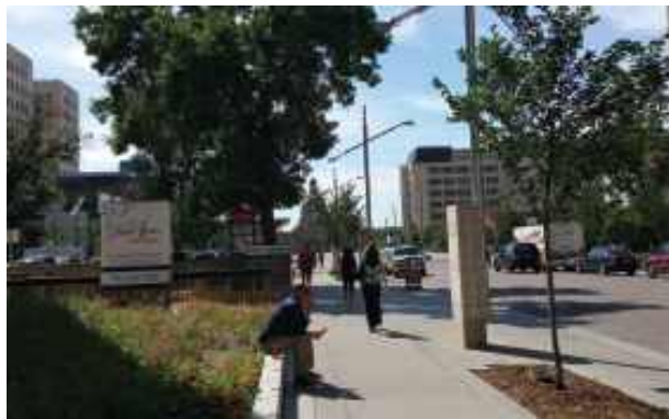
Pre-cast concrete pavers provide a durable surface for snow clearing and mulch around newly planted trees protects their root balls from compaction.
