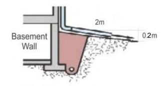
Proper grade and downspout extensions will prevent water from seeping into your foundation.
