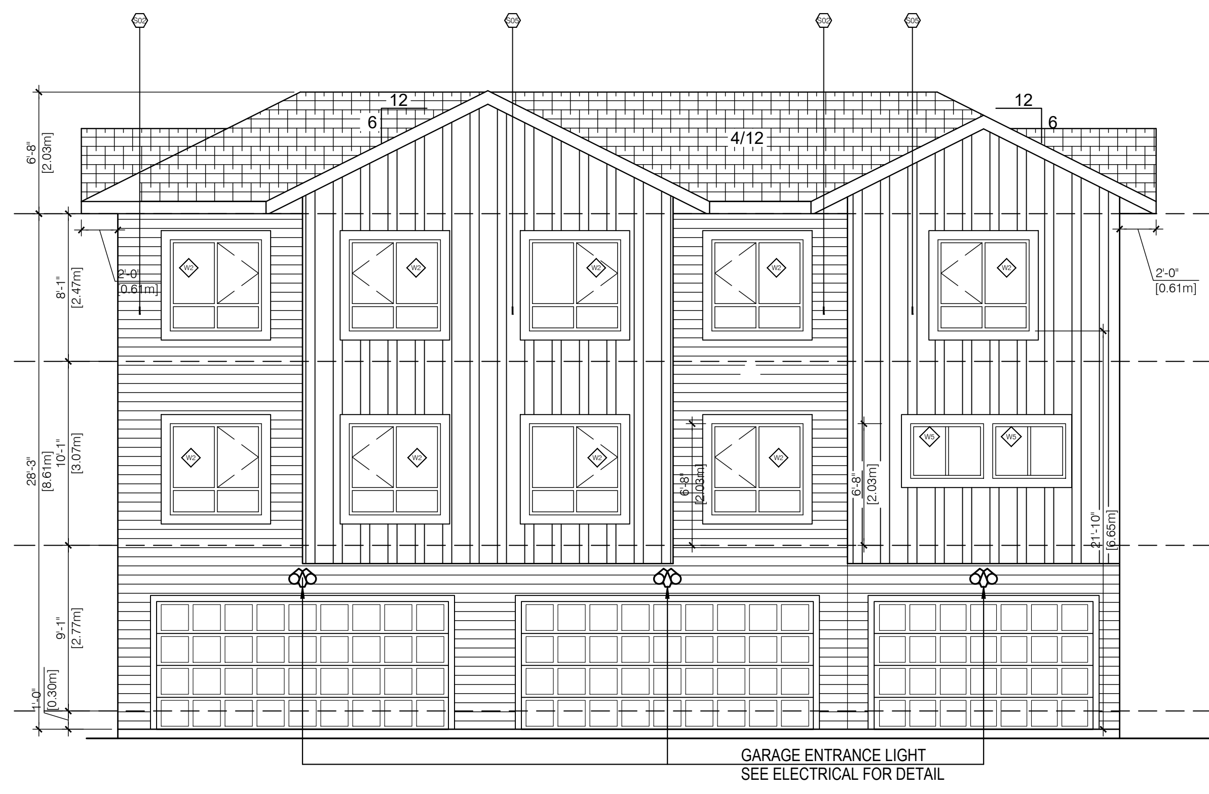
1 REAR ELEVATION ( PROPOSED ) A4.1 3/16" = 1'-0"
